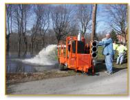
High capacity pump drains a contaminated reservoir in Indiana County.
