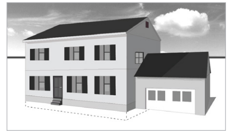
Subgrade crawlspace with attached garage
