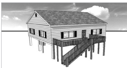
Elevated with utility chase
