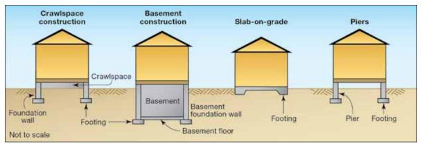
Figure 5: Examples of Foundation Types
